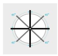
Door moves from each 45° angle, in both directions, to a hold position.
